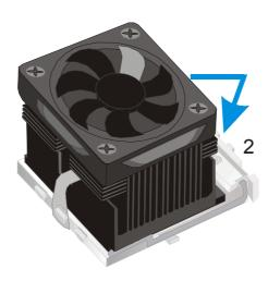
4. The fans power connector should be connected to CPUFAN1.
